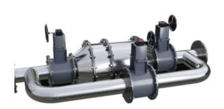
The CatEMission DPF diesel particulate filter is an essential component for the reduction of particulate matter in diesel engine exhaust gases. It operates by physical filtration, employing a "wall flow" filter design, effectively capturing soot particles that the DOC diesel oxidation catalyst is not oxidized in.
